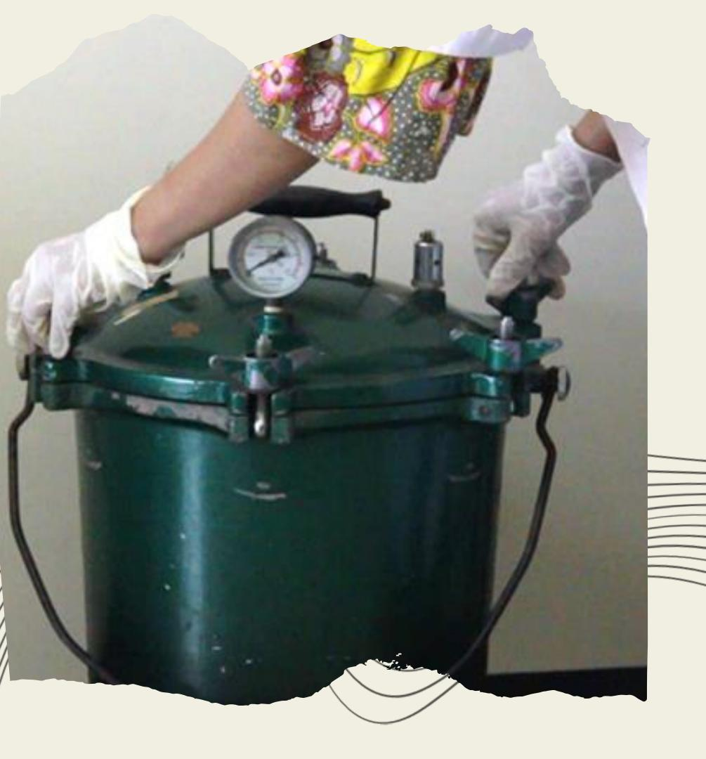
sterilized the media for 1 hour using Autoclave
