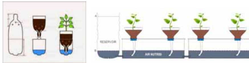
Figure 2. Wick System/ Static Solution Culture
